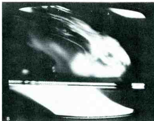
Fig. 2 Open AGC line electrolytic shown in (A) permits AGC overload (B), but sync symptom is most important clue in this kind of stage. Waveform in (C) was taken across AGC capacitor while symptom was present. Shock healed the dielectric of the electrolytic, and made the waveform normal (D).
