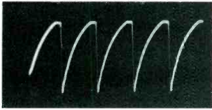
Fig. 2 Normal drive waveform on the grid of the horizontal output stage.
