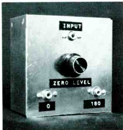
Fig. 6 The completed "two-signal" adapter, labelled for use in tracing separation problems.
